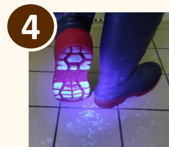
Visualisation under UV light of the « contamination » after changing zone
